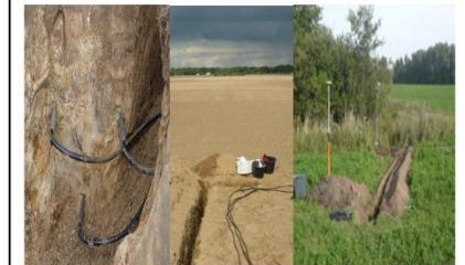
Soil moisture station set-up
