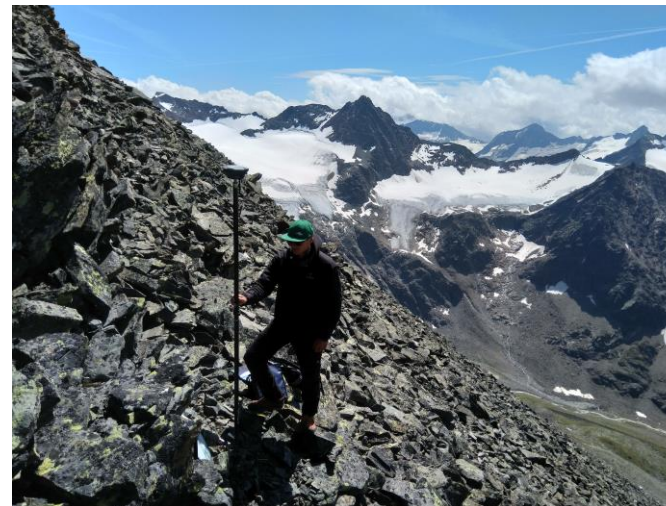
GNSS-Measurement of logger position (Image: Andreas Mayr)
